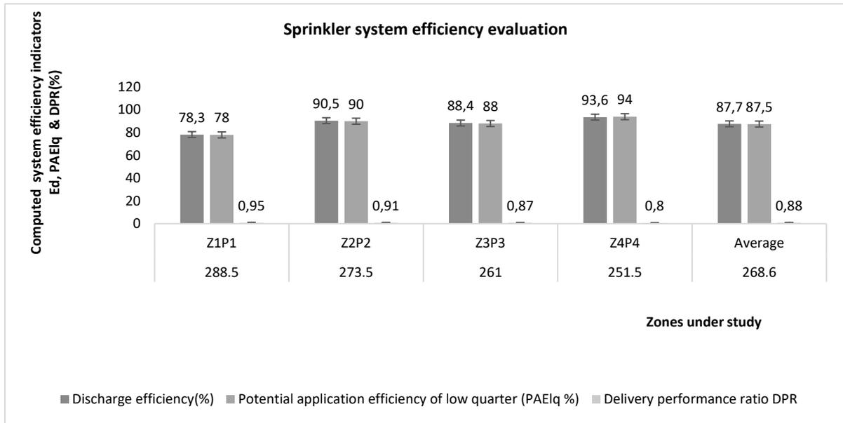
Figure 3. Computed efficiency indicators in different zones under study
