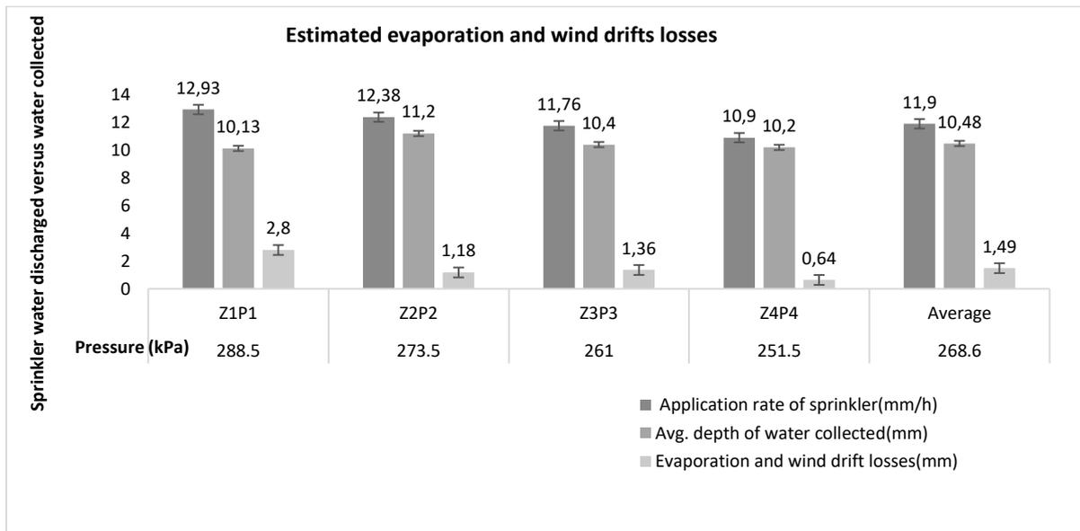
Figure 4. Estimated evaporation and wind drifts losses
