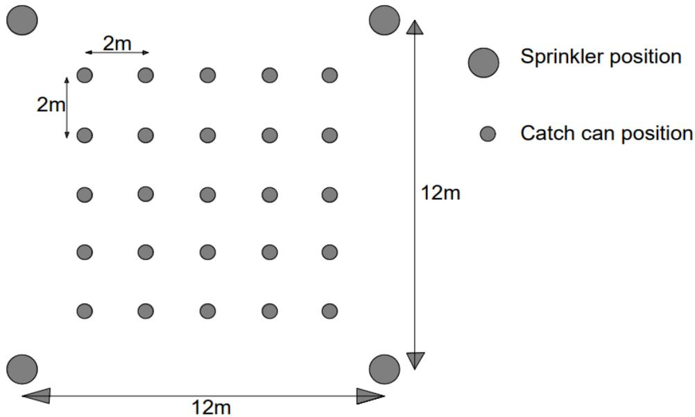
**Figure 1.** Sprinkler catch-can pattern
